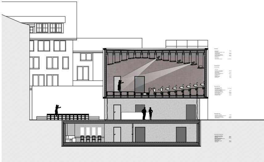
Architectural section drawing showing a cantilevered upper floor. The drawing includes a ground floor with a reception area and a first floor with a large cantilevered space containing a stage and seating. To the right, there are technical specifications and a table of dimensions.
